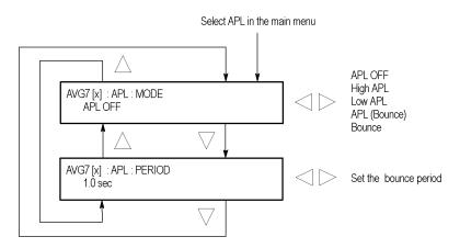
Figure 3-25: AVG7 module APL submenu
