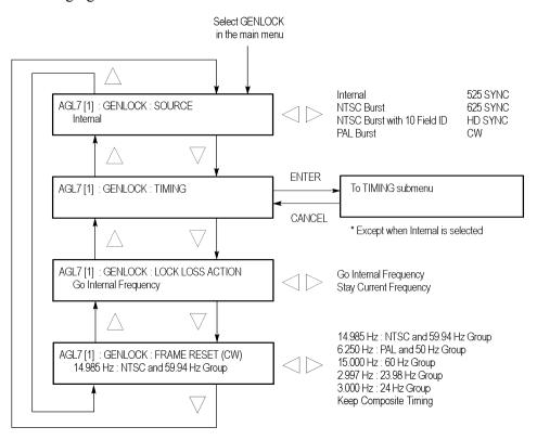
Figure 3-5: AGL7 module GENLOCK submenu
