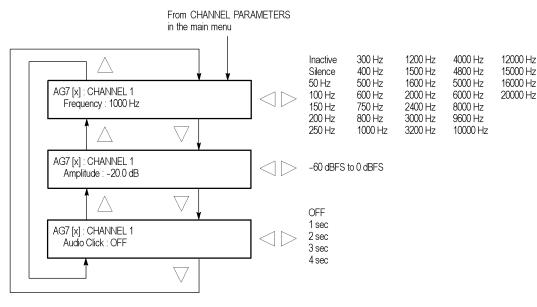
Figure 3-2: AG7 module CHANNEL PARAMETERS submenu
