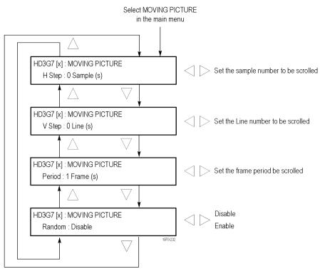
Figure 3-85: HD3G7 module MOVING PICTURE submenu
