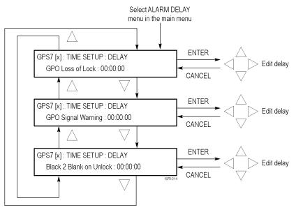
Figure 3-69: GPS7 module ALARM DELAY submenu
