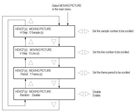
Figure 3-102: HDVG7 module MOVING PICTURE submenu
