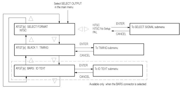
Figure 3-11: ATG7 module SELECT OUTPUT submenu
