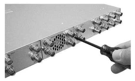
Figure 1-6: Securing the module
