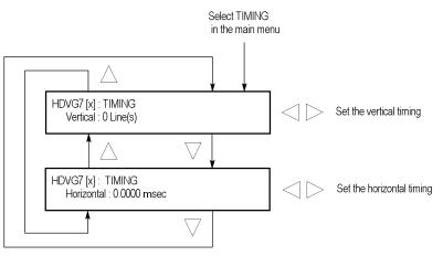
Figure 3-109: HDVG7 module TIMING submenu
