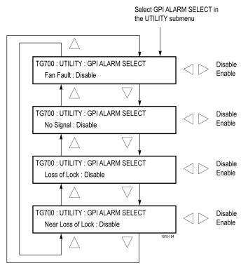
The GPI ALARM SELECT submenu contains the following selections:
