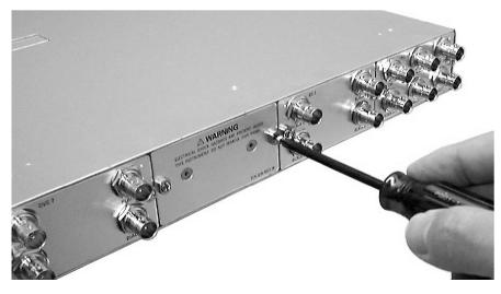
Figure 1-4: Removing the blank panel
