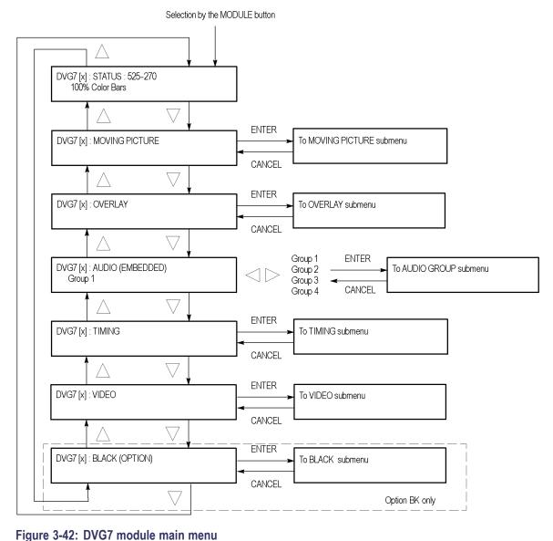
**MOVING PICTURE.** Scrolls the active picture area of the output test signal. Select this menu item, and then press the **ENTER** button to access the MOVING PICTURE submenu. (See page 3-81.)
