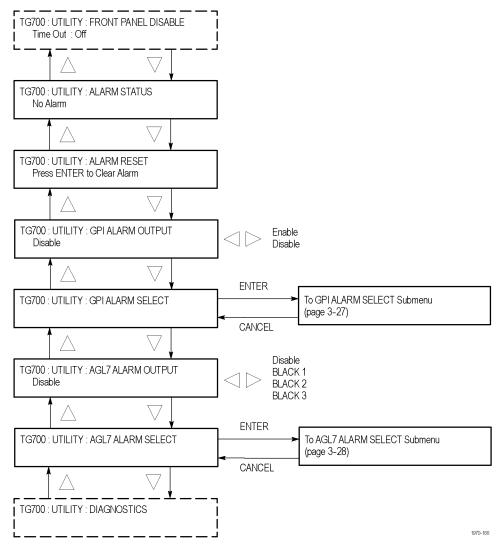
Figure 2-31: Mainframe GPI ALARM menu
