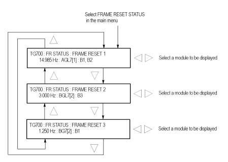
Figure 2-19: FRAME RESET STATUS submenu
