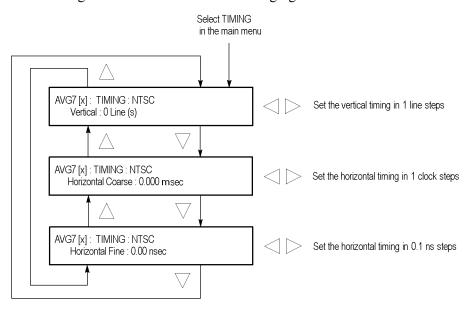
Figure 3-23: AVG7 module TIMING submenu
