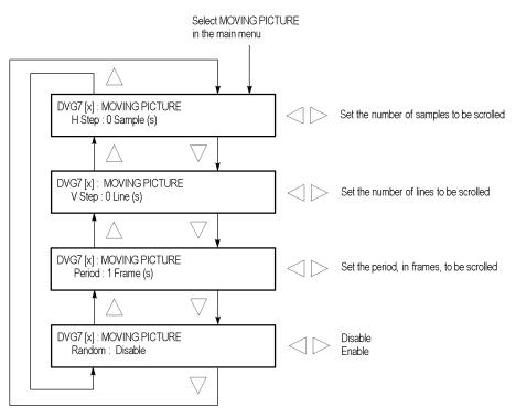
Figure 3-43: DVG7 module MOVING PICTURE submenu
