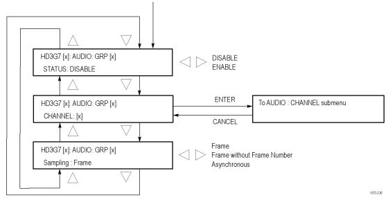
Figure 3-86: HD3G7 module AUDIO (EMBEDDED) submenu
