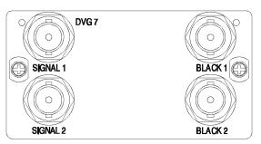
Figure 2-11: DVG7 module connectors (Option BK)
