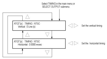
Figure 3-14: ATG7 module TIMING submenu
