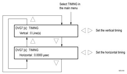
Figure 3-50: DVG7 module TIMING submenu
