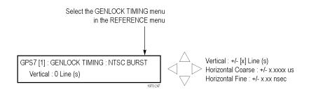
Use the up ( $\blacktriangle$ ) or down ( $\triangledown$ ) arrow button to select a timing parameter, and then use the left ( $\blacktriangleleft$ ) or right ( $\triangleright$ ) arrow button to adjust the parameter.
