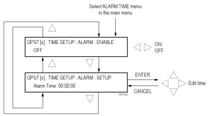
Figure 3-68: GPS7 module ALARM TIME submenu
