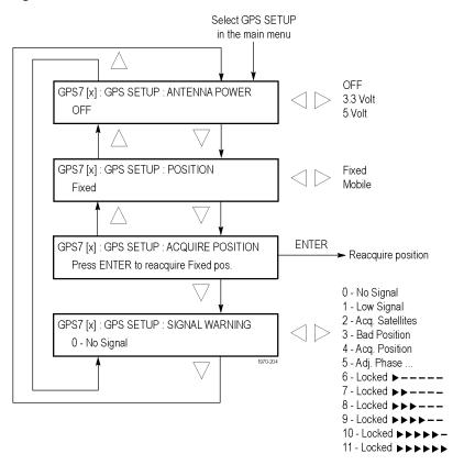
Figure 3-61: GPS7 module GPS SETUP submenu
