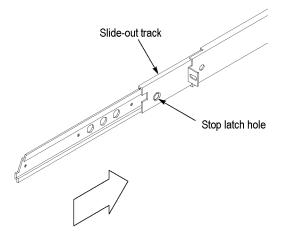
Figure 1-2: Placing the TG700 in the rack
