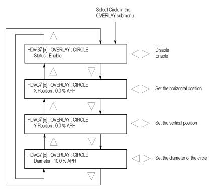
Figure 3-106: HDVG7 module CIRCLE submenu
