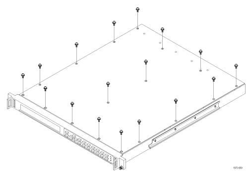
Figure 2-28: Top cover removal
