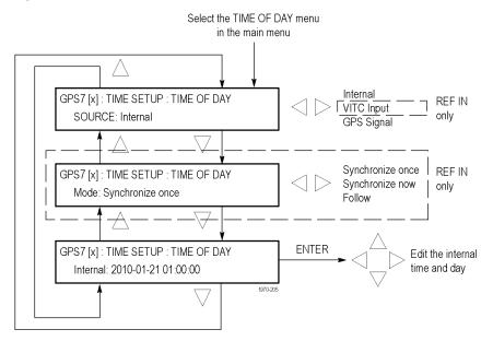
Figure 3-62: GPS7 module TIME OF DAY submenu
