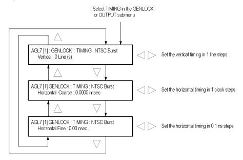
Figure 3-8: AGL7 module TIMING submenu
