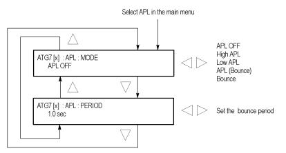
Figure 3-15: ATG7 module APL submenu
