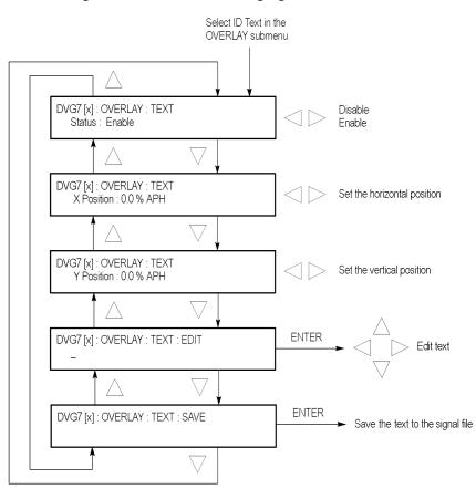
Figure 3-46: DVG7 module ID TEXT submenu
