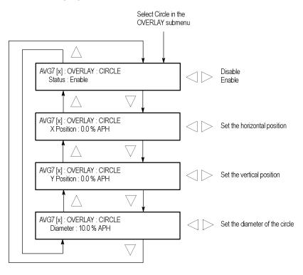
Figure 3-22: AVG7 module CIRCLE submenu
