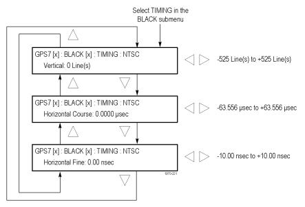
Figure 3-58: GPS7 module TIMING submenu
