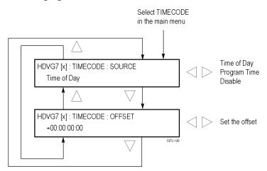
Figure 3-110: HDVG7 module TIMECODE submenu
