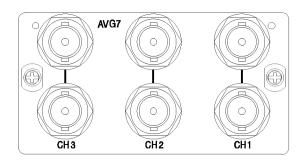
Figure 2-8: AVG7 module connectors
