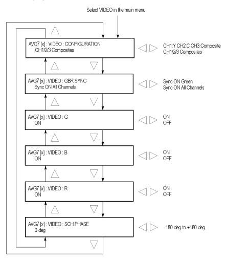
Use the up ( $\blacktriangle$ ) or down ( $\blacktriangledown$ ) arrow button to scroll through the menu. The following figure shows the VIDEO submenu.
