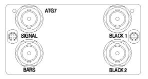
Figure 2-7: ATG7 module connectors
