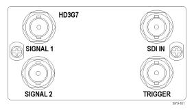
Figure 2-13: HD3G7 module connectors
