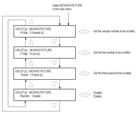
Figure 3-99: HDLG7 module MOVING PICTURE submenu
