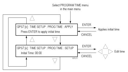
Figure 3-65: GPS7 module PROGRAM TIME submenu
