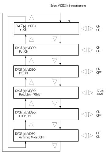
Use the up ( $\blacktriangle$ ) or down ( $\blacktriangledown$ ) arrow button to scroll through the menu. The following figure shows the VIDEO submenu.
