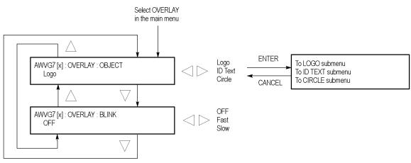
Figure 3-29: AWVG7 module OVERLAY submenu
