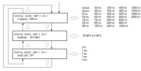
Figure 3-49: DVG7 module AUDIO CHANNEL submenu
