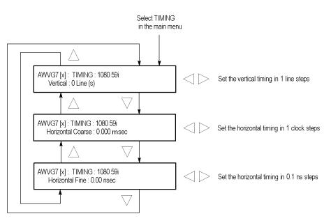
Figure 3-33: AWVG7 module TIMING submenu
