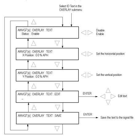
Figure 3-31: AWVG7 module ID TEXT submenu
