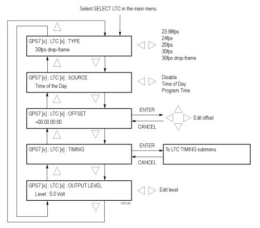
Figure 3-70: GPS7 module LTC submenu
