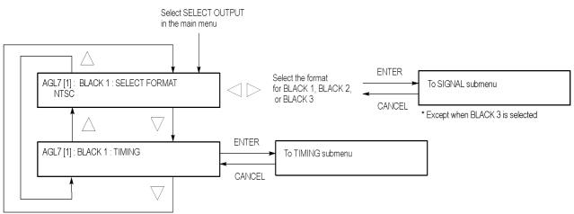
Figure 3-6: AGL7 module OUTPUT submenu
