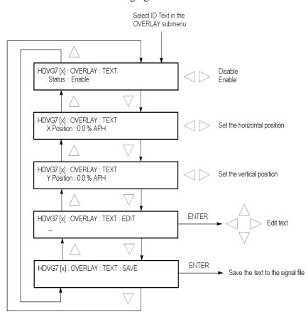
Figure 3-105: HDVG7 module ID TEXT submenu
