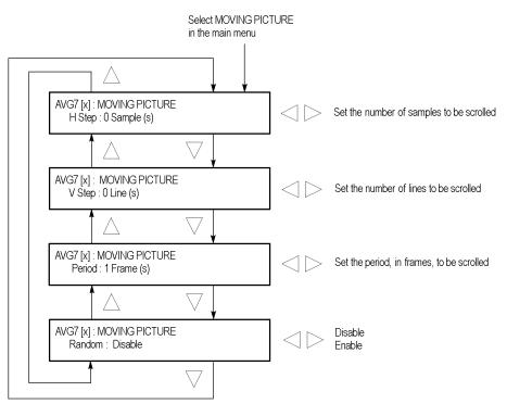
Figure 3-18: AVG7 module MOVING PICTURE submenu
