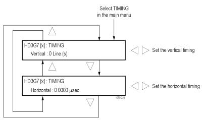
Figure 3-88: HD3G7 module TIMING submenu
