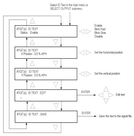
Figure 3-13: ATG7 module ID TEXT submenu
