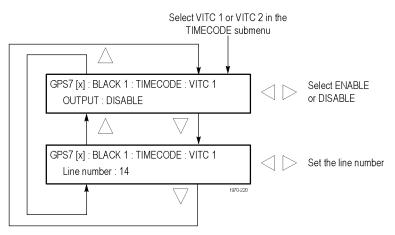
Figure 3-60: GPS7 module VITC submenu
