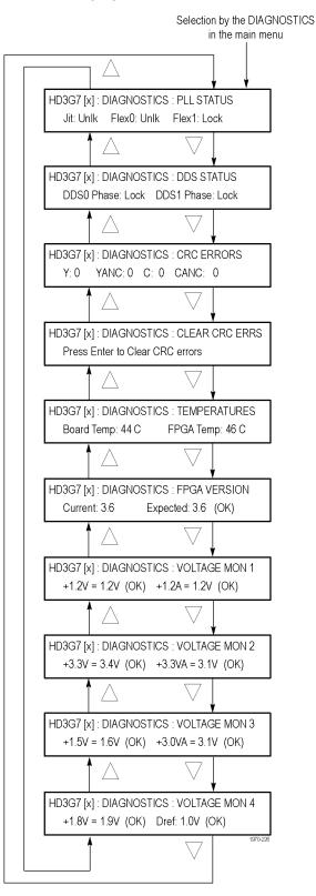
Figure 3-95: HD3G7 module DIAGNOSTICS submenu
