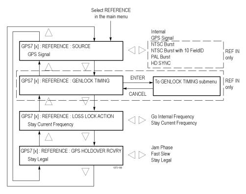
Figure 3-56: GPS7 module REFERENCE submenu
