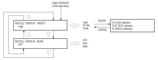
Figure 3-19: AVG7 module OVERLAY submenu
